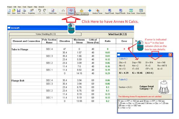
When a parameter exceeds the limiting value in Annex N, the software sets the value of that parameter to the limiting value in Annex N
